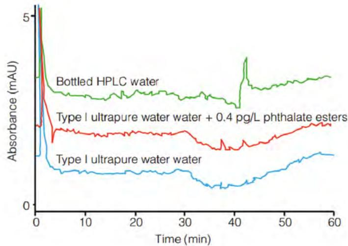
**Figure 1.** A comparison of purified water qualities used in HPLC. 50 ml water concentrated on a C18 column and eluted with a water:acetonitrile gradient, 0–100% at 5%/min, flow rate 2 ml/min, with UV detection at 254 nm.<sup>9</sup>
