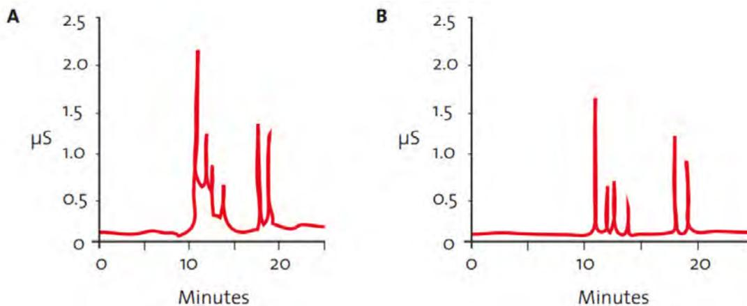
**Figure 2.** The effect of ionic contaminants from water on baseline used in ion chromatography, integration and resolution: (A) poor water quality and (B) Type I (18.2 MΩ-cm) water. The ‘noise’ introduced around the 10–15 minute mark is clearly apparent.<sup>10</sup>
